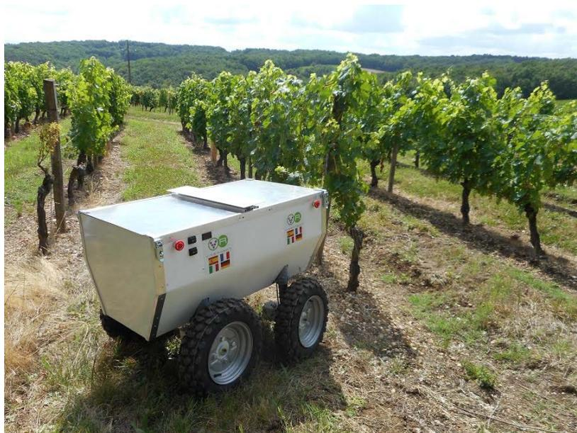
*Figure 3. Images of the first prototype of the VineRobot*
